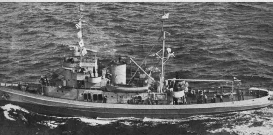
Fleet tug (AT) has several functions during an invasion. It is used to maneuver LST's or LCI's which may be damaged, fight fires, salvage small craft or go to the rescue of personnel.
